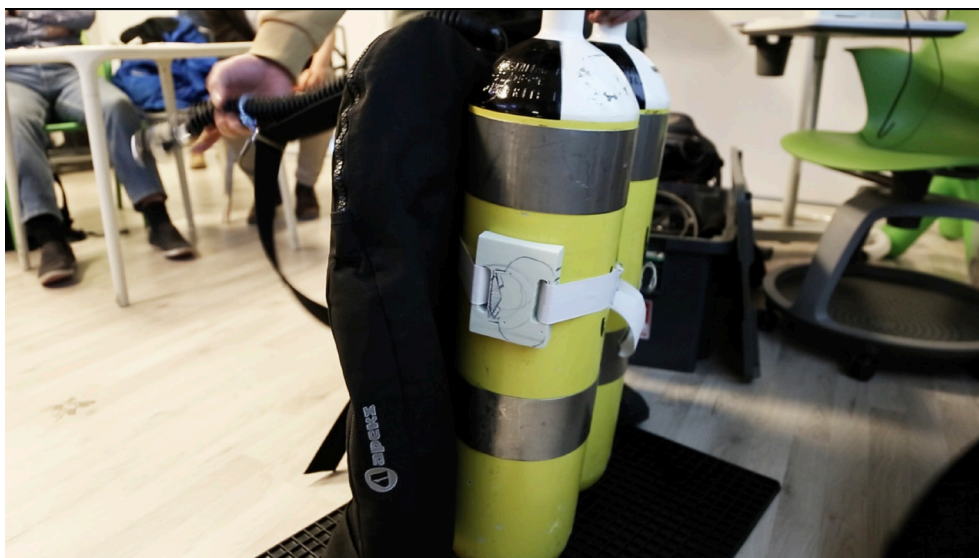
Figure 19. Mock-up of the sound emitting unit attached in air tank
