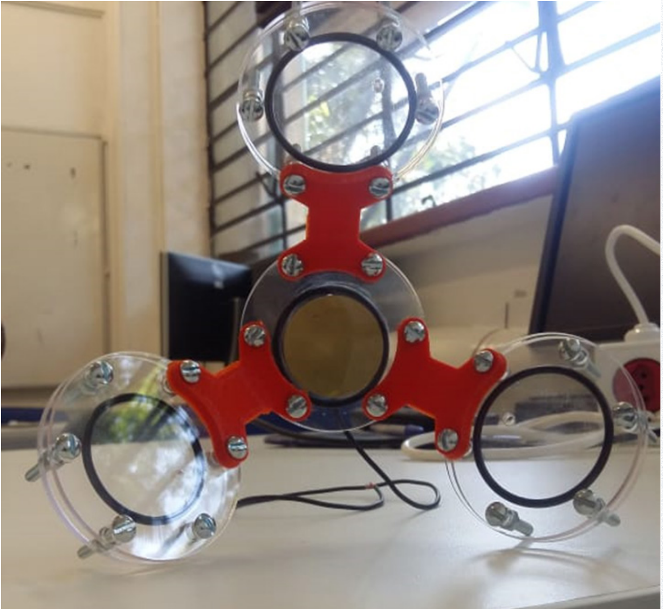
Figure 25. Structure that enables omnidirectional signals with planar piezoelectric rings
