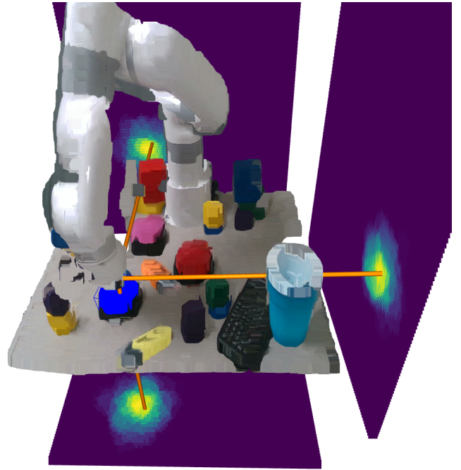
Fig. 2: Heatmap visualization of the guidance distribution, generated online by our proposed agentic framework, which produces code that biases a robot policy’s action distribution towards desirable behavior.
